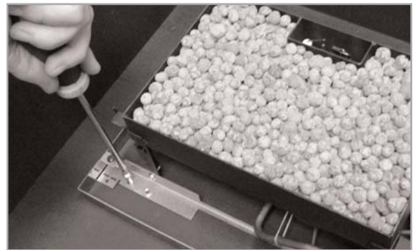
Securing the burner
